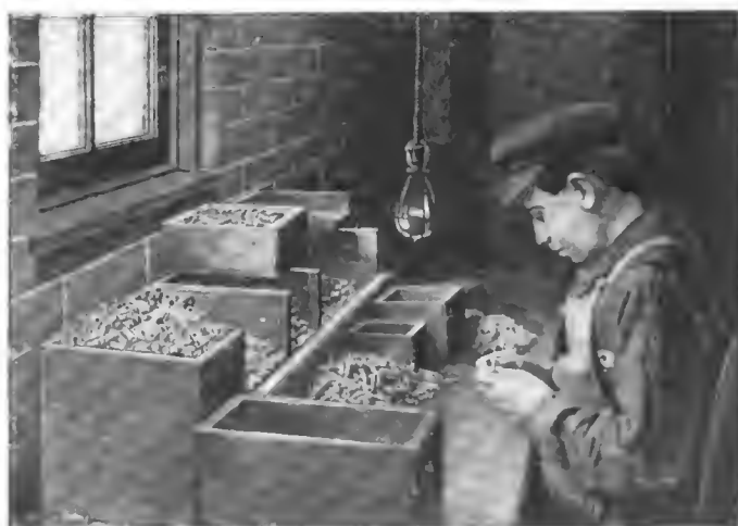
SORTING TIMKEN ROLLERS AFTER THE FIRST GRINDING.
